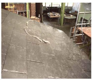
There is currently no British Standard test for driving rain testing. The State vent range has been tested at the Building Research Establishment for rain penetration. Test results and methods are available on request.
